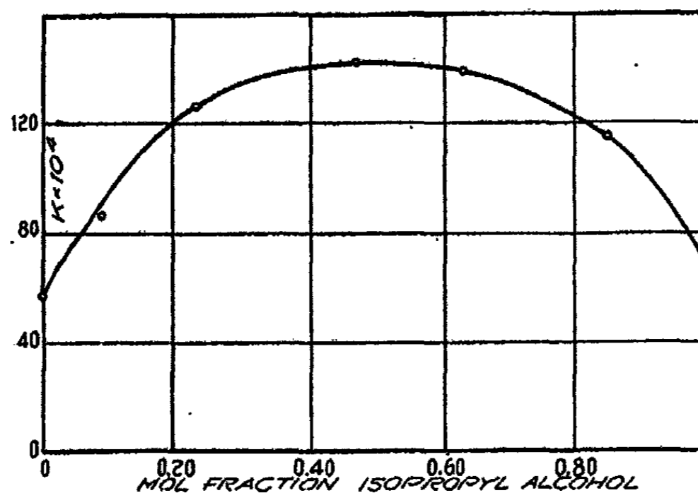
FIG. 1 Reaction rate in isopropyl alcohol-water solutions at 40°C.
